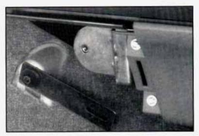
Loosen the nut and move the bracket out of the way.
